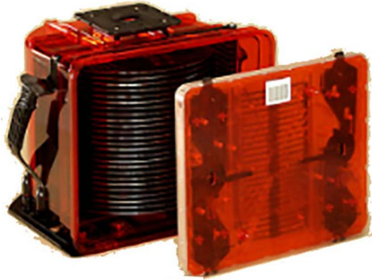
Figure 22: A FOUP With Wafers
