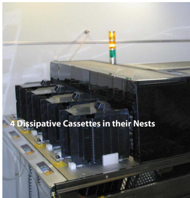
Figure 19: An Open Cassette Tool With Four Dissipative Cassettes Loaded
