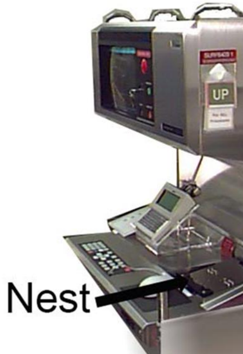
Figure 18: An Open Cassette Process Tool Input Port
