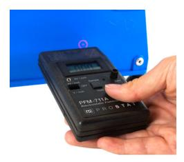
Figure 2. An electrostatic fieldmeter measuring at 1" from a surface. Photo courtesy of Prostat Corporation.
