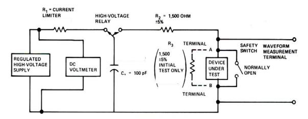
Figure 1: HBM Circuit Schematic MIL STD 883, Method 3015.2
