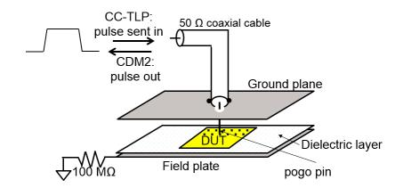
Figure 4: Conceptual illustration of CC-TLP and CDM2. Both use a relay to initiate a square transmission line pulse through a 50  $\Omega$  system.
