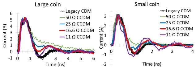
Figure 6: A comparison of the discharge waveforms from the legacy CDM tester and CCDM testers of various system impedances. Calibration coins are used as the DUT.
