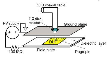
Figure 1: Illustration of the CDM tester used in the ANSI/ESDA/JEDEC standard.
