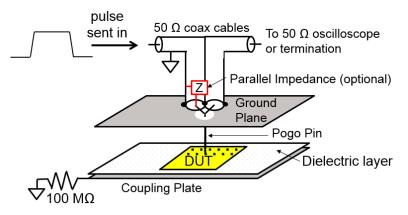
Figure 5: Illustration of low-impedance contact CDM. Parallel impedances in the pulse delivery network reduce the system impedance below 50  $\Omega$ .
