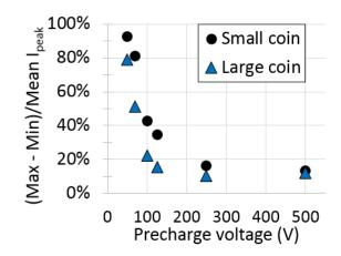
Figure 2:  $I_{peak}$  maximum - minimum (top) and the standard deviation (bottom) of 50 zaps to JEDEC calibration coins as a percentage of the mean; 26% relative humidity. Data taken using an 8 GHz oscilloscope.
