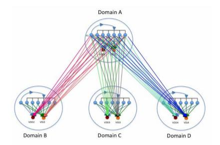
*Figure 1* shows a simple case where 7-pins must be stressed to their local power and ground pins in domain A and again for three additional supply domains, B, C and D.
