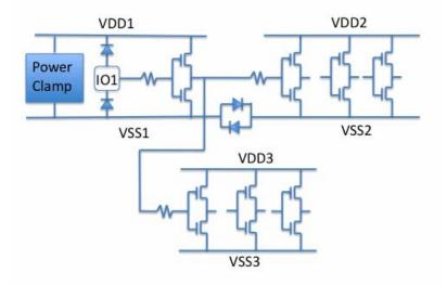
Figure 2 shows a schematic of an input signal from power domain 1 (VDD1) to CMOS inverters in power domain 2 (VDD2) and power domain 3 (VDD3).
