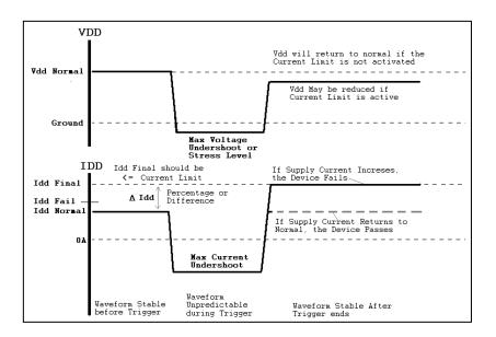
Figure 7: Example of Latch-up failure using Combined Bias/Stimulus TLU (Idealized Oscilloscope Graph)
