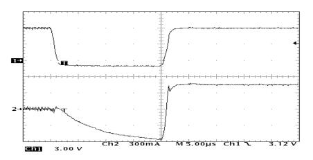
Figure 8: Example of Latch-Up failure using Combined Bias/Stimulus TLU (Actual Oscilloscope Plot)
