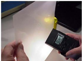
Fig. 5 Charged page protector reading negative 10,320 volts
