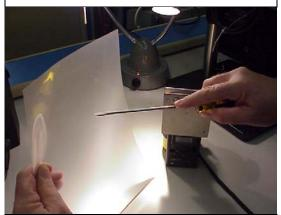
Fig. 7 Screwdriver blade momentarily grounded by the operator's index finger with the blade tip about an inch away from the page protector (the operator is wearing a wrist strap)
