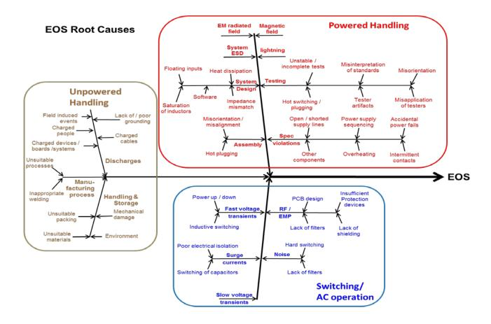
Figure 4: "Fishbone" Diagram Indicating Categorization of EOS Root Causes<sup>2</sup>
