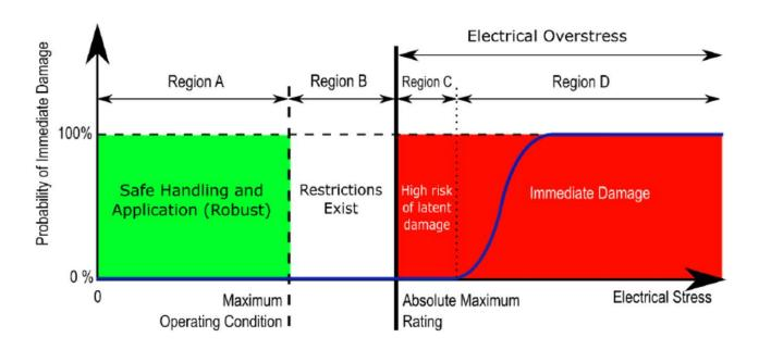
Figure 5: A graphical depiction of how Absolute Maximum Ratings should be interpreted. The blue line is the number of components suffering immediate, catastrophic EOS damage.
