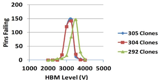
Figure 1: Distribution of HBM failure voltages for identical pins. Typical behavior is shown on the left side denoting the important parameters. Actual measured failure distributions from three different sets of clones are shown on the right side for three different products with cloned IO pins.
