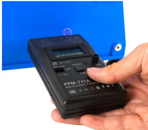
Figure 2. An electrostatic fieldmeter measuring at 1" from a surface. Photo courtesy of Prostat Corporation.
