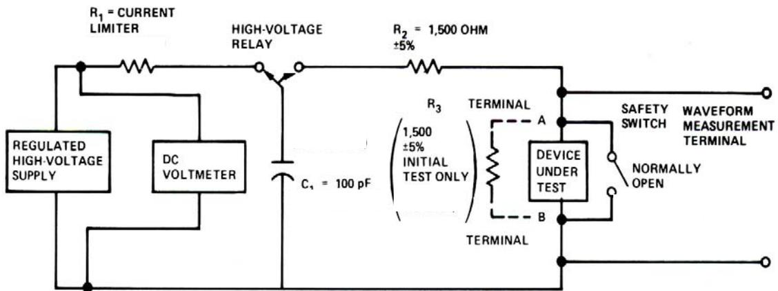
Figure 1: HBM Circuit Schematic MIL STD 883, Method 3015.2
