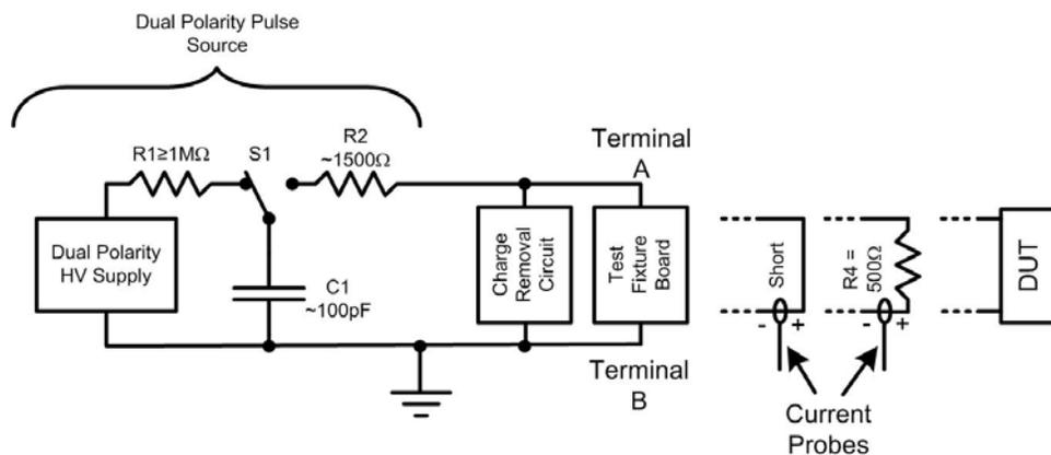
Figure 2: HBM Circuit Schematic in Merged ESDA/JEDEC Standard
