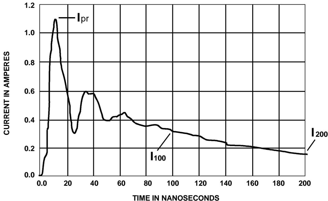
**Figure 1: Current MM waveform through a 500 ohm resistor for a 400 volt discharge**
