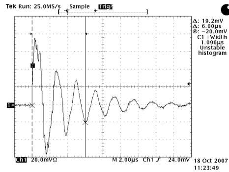
Discharge from a 1 meter cable charged to about 300V.
