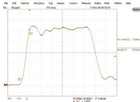
In practice, an air breakdown between the cable and its mating connector is likely prior to a hard contact being made; an arc occurs resulting in a fast transient current spike being injected.
