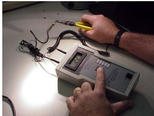
Fig. 4 Needle nose pliers with a system resistance of  $2.29 \times 10^6$  ohms (borderline conductive and OK)
