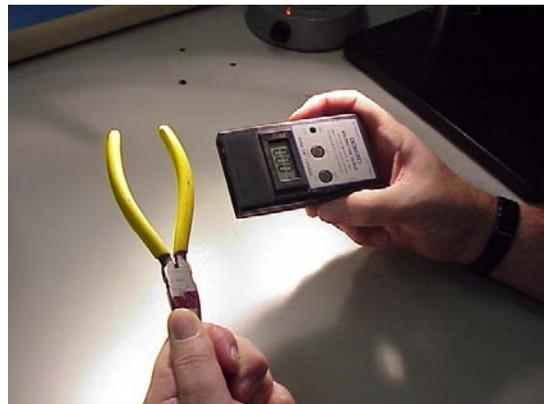
Fig. 2 Grips on needle nose pliers with no measurable field strength
