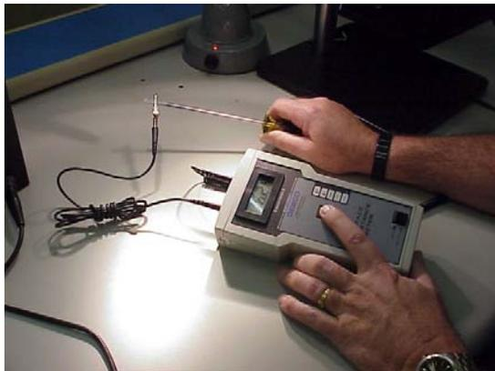
Fig. 3 Screwdriver with a system resistance of  $6.21 \times 10^{12}$  ohms (insulative – charge will not flow to ground)
