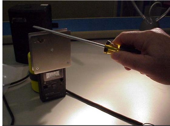
Fig. 6 Insulative handled screwdriver with a 20 volt charge (meter wasn't accurately brought to a zero reading)
