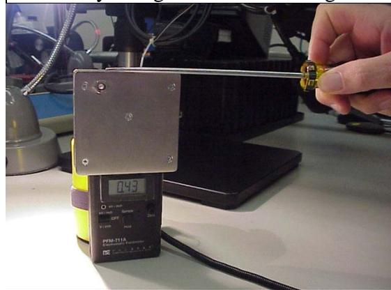
Fig. 8 Screwdriver blade with CDM charge immediately brought in contact with the charge plate and the resulting 430 volts of CDM discharge - That is significant!
