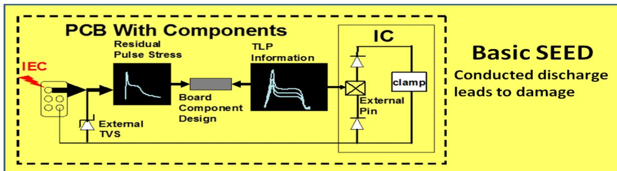
Fig. 3: The new accepted understanding of the impact on manufacturing corresponding to the component IC's HBM level. The residual pulse after external clamp is matched with the TLP information of the interface IC pin for different time domains. The board components are tuned for robust IEC protection.
