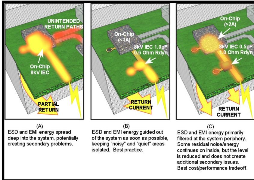
Fig. 4: Discharge paths through a wired network showing the different strategies. On-chip protection for system level ESD does not yield optimum results.
