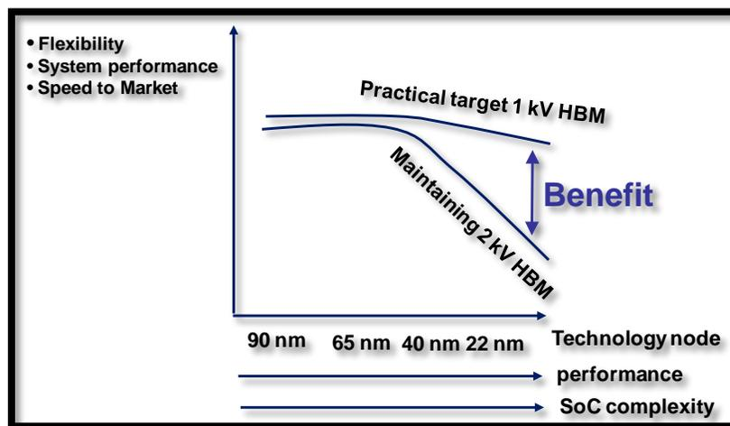
Fig. 2: Changing from 2kV HBM target to the more-than-safe 1kV HBM facilitates the important advantage of meeting high-speed requirements. It has benefits to both the OEM and the IC supplier of enabling delivery of high performance products with advanced technologies on time.
